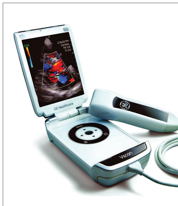
GE's Vscan ultra-portable ultrasound produces images in real time
