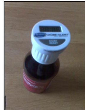
Figure 2: Dose-alert Low-Cost Electronic Medication Reminder
