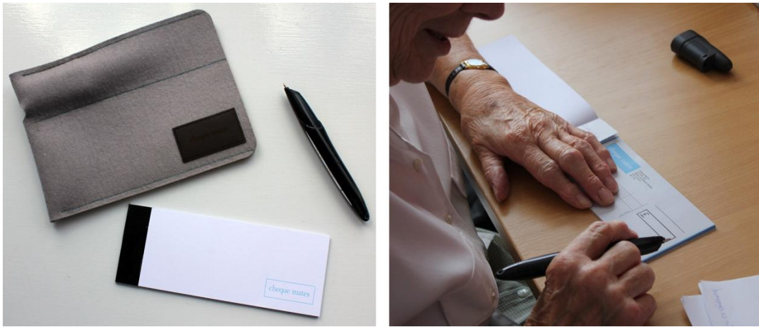
Electronic pen and cheque book. Here the Anoto R pen senses what you write and transmits the information to the payment system.
