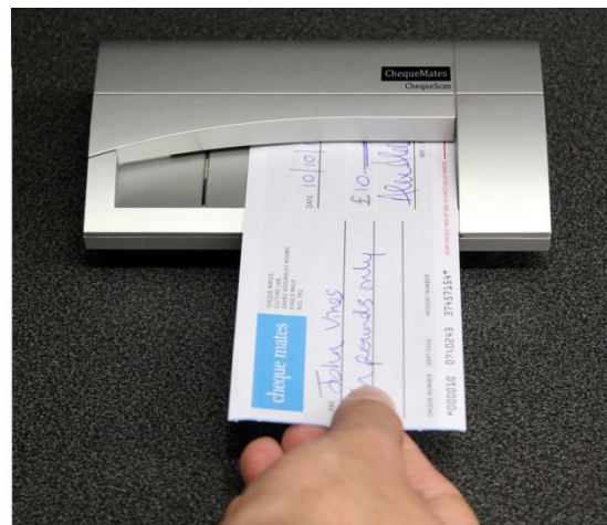
Cheque scanner and cheque book. Payer writes a cheque. This is scanned by the payer or the payee to initiate an electronic transaction.
